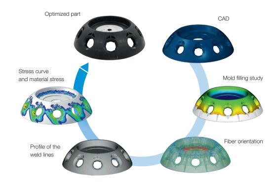
Fig. 10: Process of designing parts with the BASF simulation tool Ultrasim®
