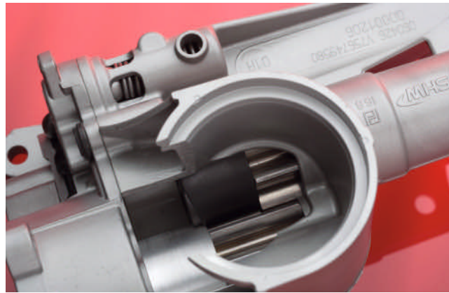
Fig. 3. Oil pump piston from SHW (Schwäbische Hüttenwerke Automotive): A BASF polyethersulfone specially optimized for dynamic friction properties soon will be officially adopted into the range under the name Ultrason E 2010 C2 TR (TR: tribology); its wear rate – without the use of lubricant – is several hundred times that of traditional PESU
