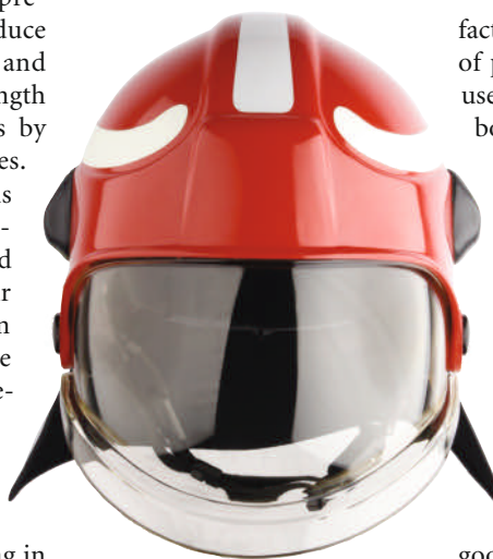
Fig. 10. The visor of the firefighter's helmet is made of the high-transparency PESU variant Ultrason E 2010 HC. The combination of high heat resistance, inherent fire retardancy, high transparency and break resistance are exploited here. These special grades feature significantly reduced inherent yellowness, thereby achieving high optical purity
