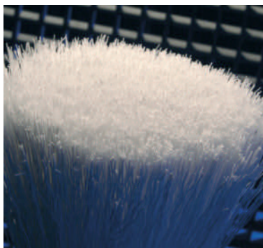
Fig. 8. Precipitated polyarylsulfones have pores with very easily controllable, low diameters, and are increasingly used in the micro and ultrafiltration, as in the hollow fiber bundle shown here. The high thermal and hydrolysis resistance permits repeated sterilization
