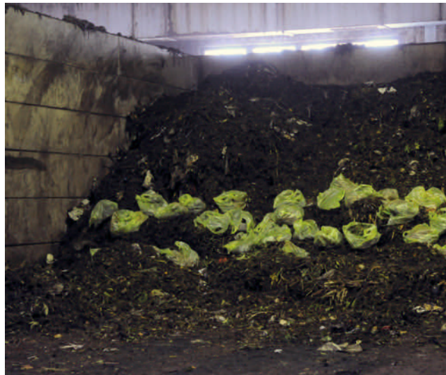
Fig. 5. In the organic refuse composting facility in Grünstadt (Rhineland-Palatinate, Germany), BASF demonstrated the compostability of organic refuse bags made from the biodegradable plastic Ecovio in 2009. In 2011, a large-scale test will be conducted with 65,000 households; this test will be evaluated by the organic refuse composting facility in Grünstadt together with an independent institute (photo: BASF)
