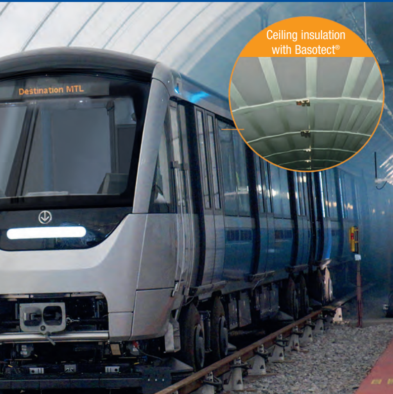
Thermal insulation and sound absorption in the ceiling area of subway cars in Montreal, Canada. Photo: Bombardier, Inc.
