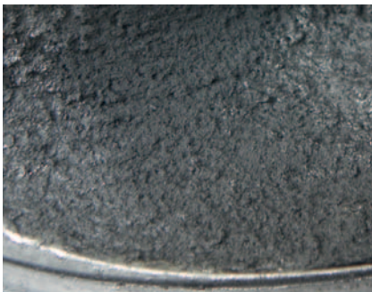
Fig. 2. Soot deposits in a polyamide charge-air duct after 30,000 km in short trips (left), possible surface defects (right)
