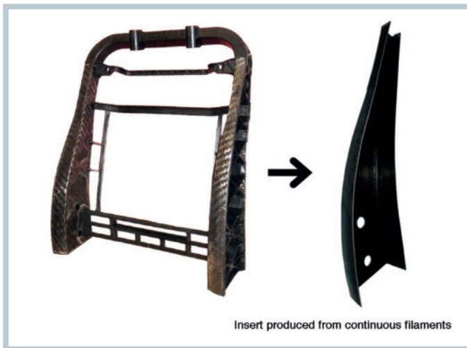
Fig. 6. Design of a seat back reinforced with inserts produced from laid continuous filaments
