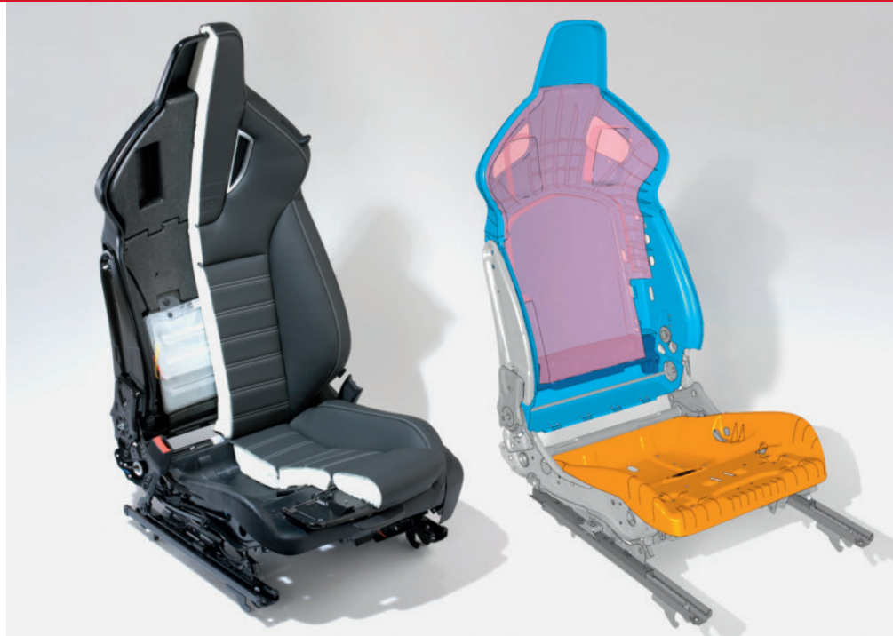
Fig. 1. Driver's seat for the Opel Insignia OPC: plastics and foams complement each other here to provide optimum crash resistance
