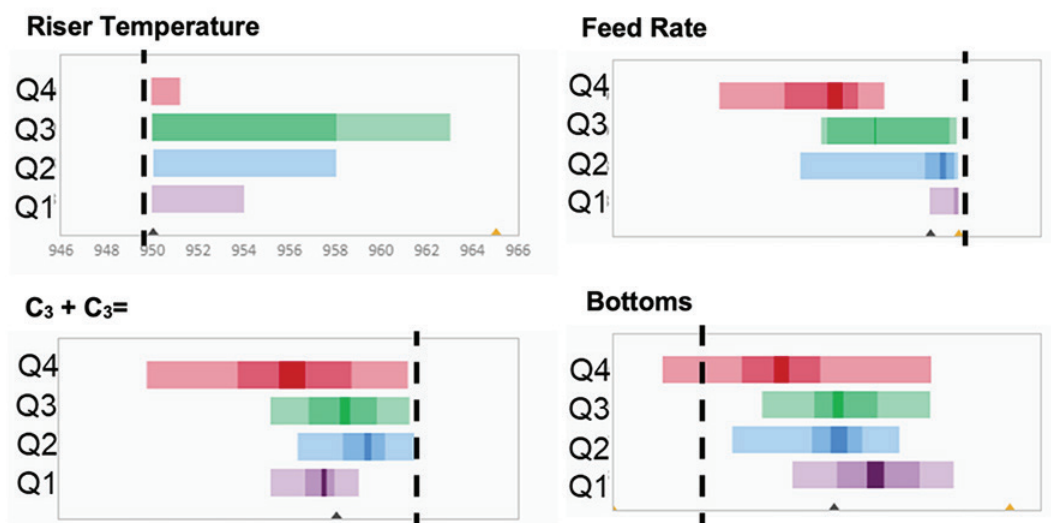
FIG. 6. FCCU operating data dashboard reveals bottoms cracking improvement opportunity due to operation against LPG constraint.
