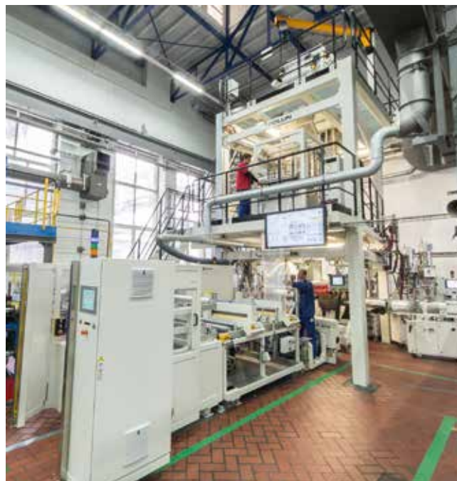
Fig. 4. Besides injection molding, extrusion is also covered in the pilot plant facility. The coextruded blown and cast film line can produce films with up to seven layers
