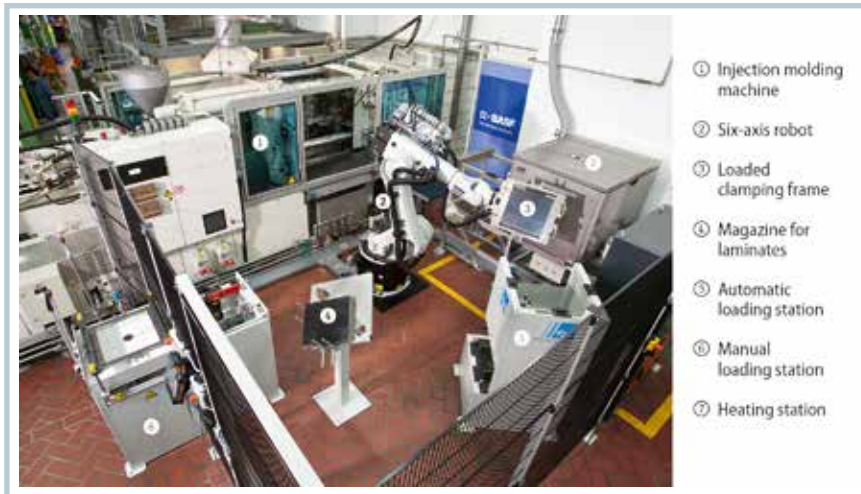
Fig. 3. The Ultracom manufacturing cell enables a fully automated process for producing thermoplastic composites within a typical injection molding cycle time to be achieved (© BASF)
