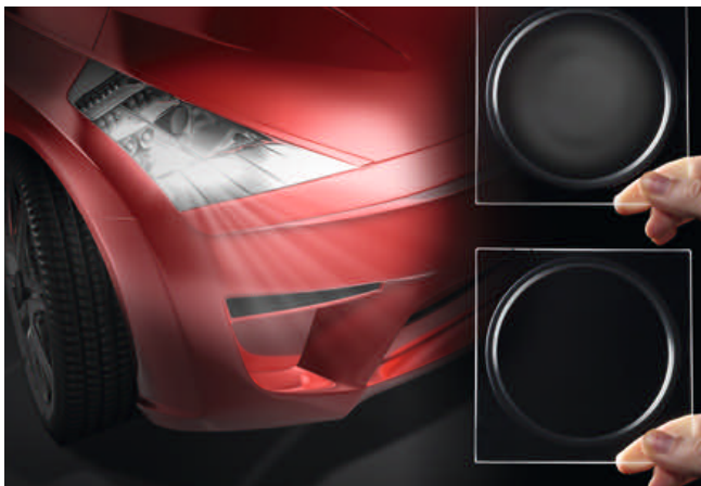
Fig. 5. High-gloss metalized headlight bezels are an important PBT application. A newly developed PBT is characterized by extremely low out-gassing in extended operation at 160 °C, whereas standard PBT can cause fogging of the headlight lens under such operating conditions
