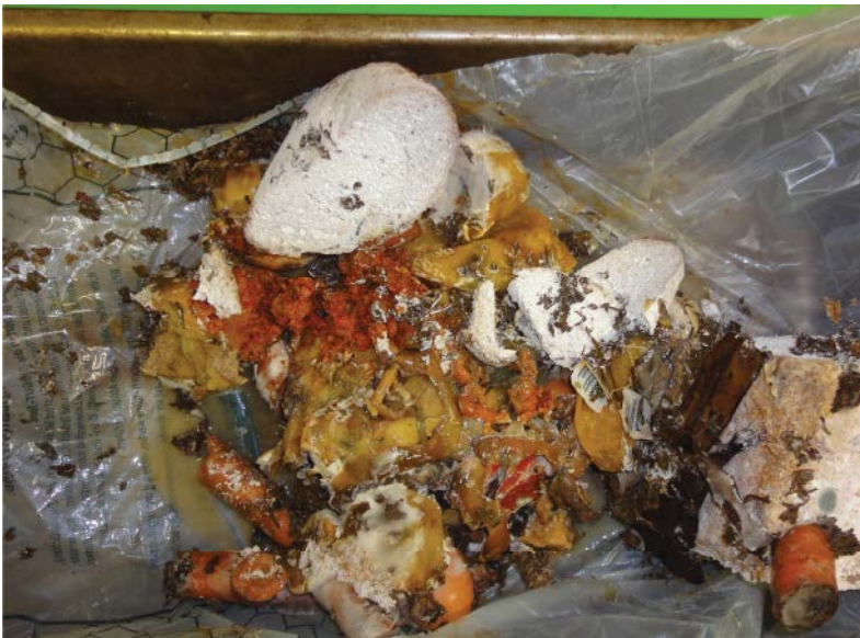
Figure 4 Kitchen waste after 14 days in an ecovio® bag with a ventilated kitchen catcher
