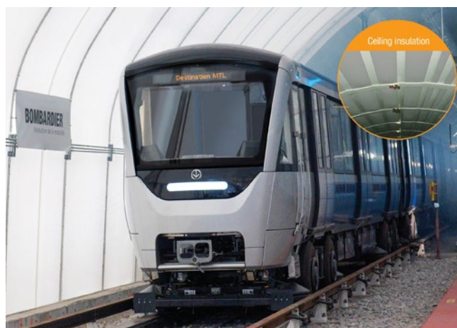
The melamine resin foam Basotect® from BASF is being used for thermal and noise insulation in the ceiling area of 468 new subway cars that Bombardier is building for the subway system in Montreal, Canada. (Photo: Bombardier, Inc., 2014)
