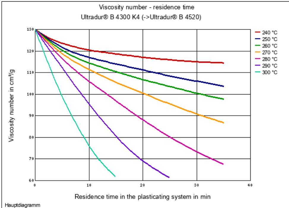
Unnecessarily high melt temperatures and excessively long residence times of the melt in the cylinder and the hot runner can bring about molecular degradation.
