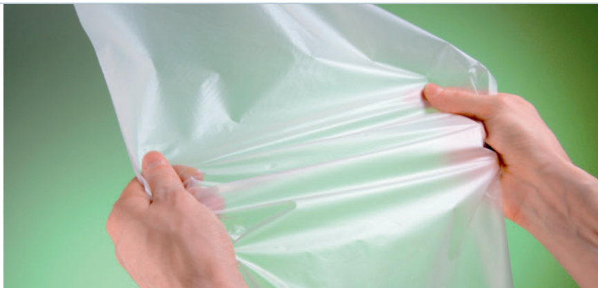
Fig. 6. Film made of Ecovio becomes waterproof and tear-resistant by its share of Ecoflex
