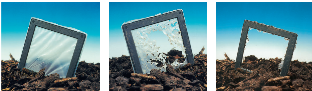
Fig. 3. Fossil-based biodegradable plastic Ecoflex satisfies the stringent requirements of the most important international standards for biodegradability and compostability: the figure shows, from left to right, decomposition of an Ecoflex film within four weeks in compost at a temperature of 55 °C
