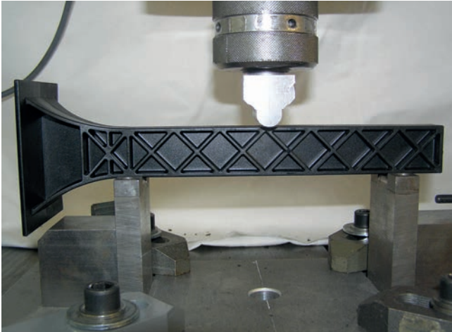
Fig. 4. A 3-point bending test showed that the maximum necessary work of fracture for Ultramid XP grades which exceeds that of comparable PA6 and PA66 grades © BASF
