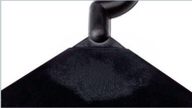
Dull spots caused by a cross section transition
