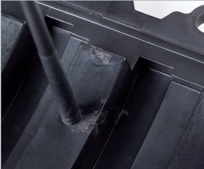
Cold slug from the bore of a machine nozzle that has cooled and broken off (glassfiber-reinforced Ultradur®)
