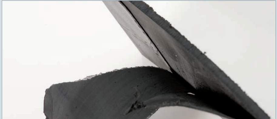
Delamination due to an injection speed that is too high (Ultramid T)
