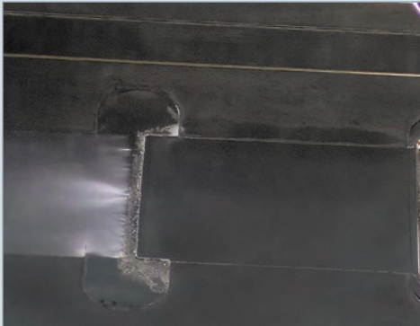
Plate-out/mold deposit at the end of the flow path due to a lack of venting
