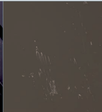
Delamination caused by entrapped air during metering (unreinforced Ultramid)
