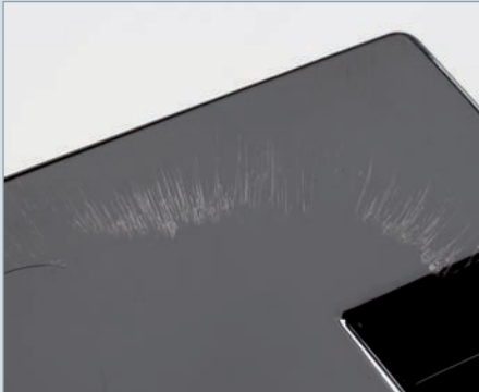
Burning streaks due to thermal degradation
