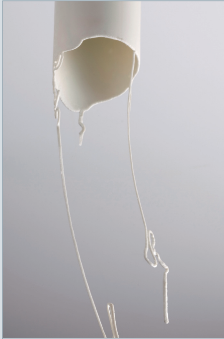
Jetting on a sleeve caused by three-fold gating through a pin gate
