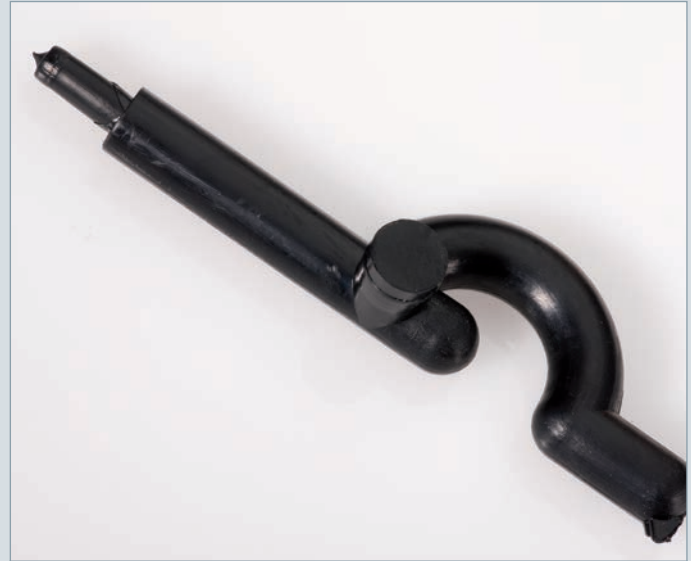
Cold slug catcher in a gate with a deflection in order to prevent jetting (injection through the parting surface)
