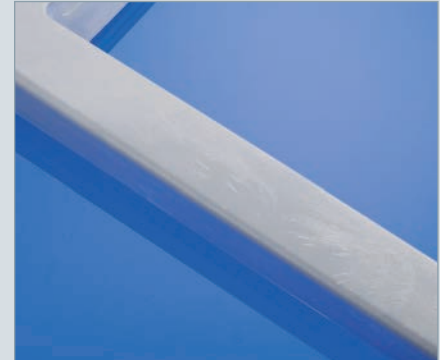
Streaks caused by thermal factors
