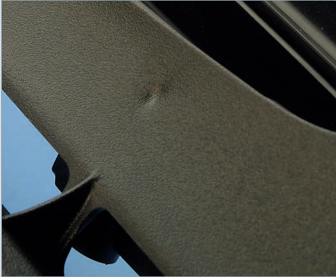
Sink mark in a section with an increase of wall thickness: the design of the screw-in mandrel is not appropriate for processing this plastic
