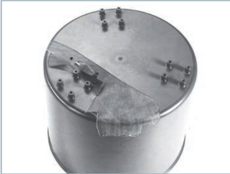
Delamination caused by an injection speed that is too high (mineral-filled Ultramid®)
