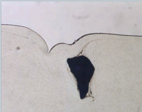
Deposits from a hot runner following a standstill of the machine (Ultrason)
