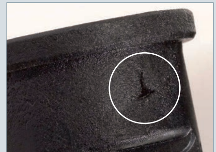
The flow pattern shows the weld lines of several melt flows.
