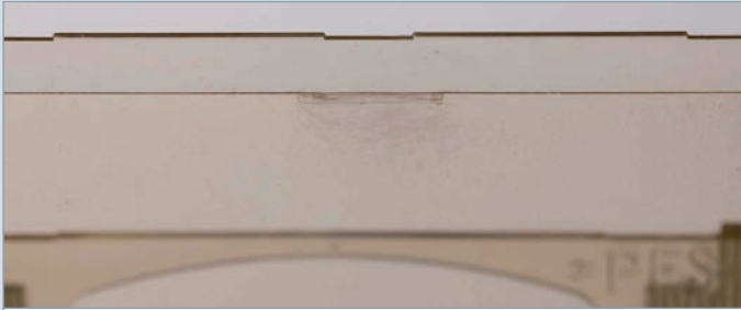
Dull spots in the area of a film gate
