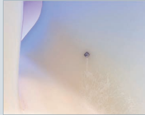
Black specks caused by foreign granules
