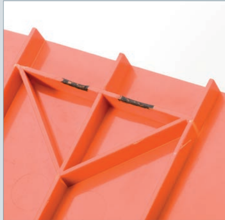
Diesel effect in a rib due to a lack of venting
