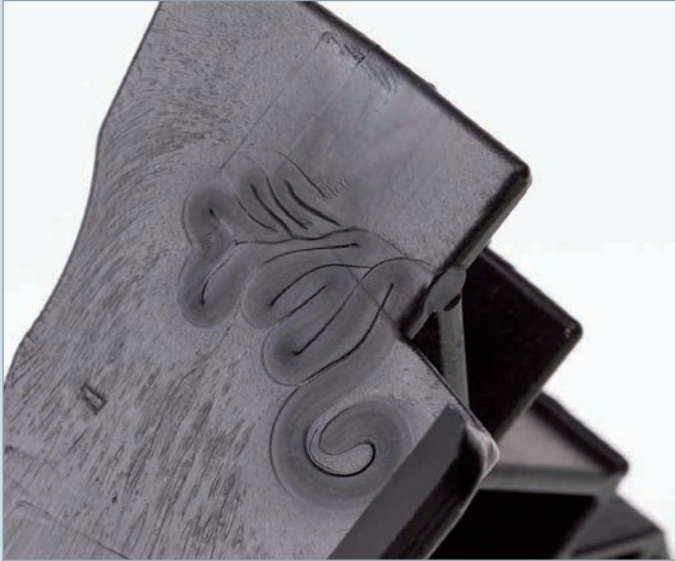
Jetting due to the unfavorable position of the gate
