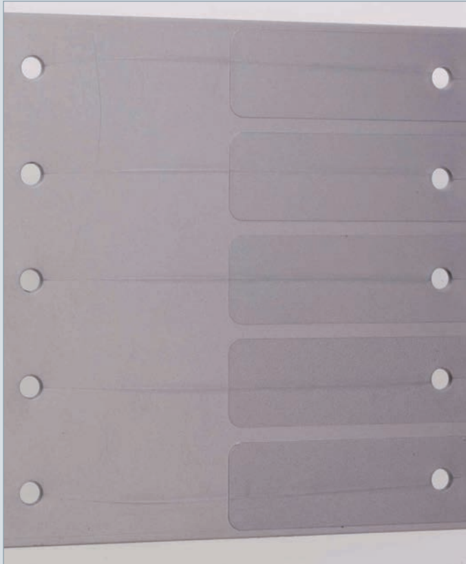
Weld lines after holes
