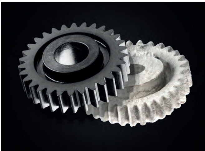
Fig. 4: Gear wheel made of Ultramid® Structure D3EG10 LFX before and after ashing.
