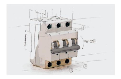
low water uptake dimensional stability hydrophobicity Polyphthalamide PPA blend or PPA copolymer, < 55% aromatic diacid content PA = Polyamide
