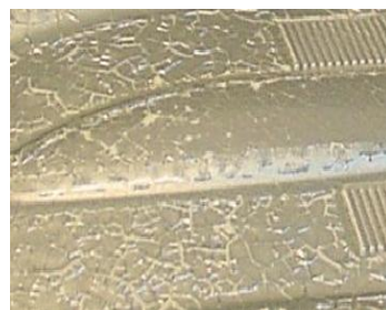
Without HALS: cracking
