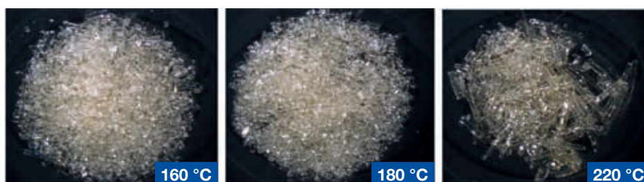
Kollidon® VA 64 extrudates obtained at different extrusion temperatures
