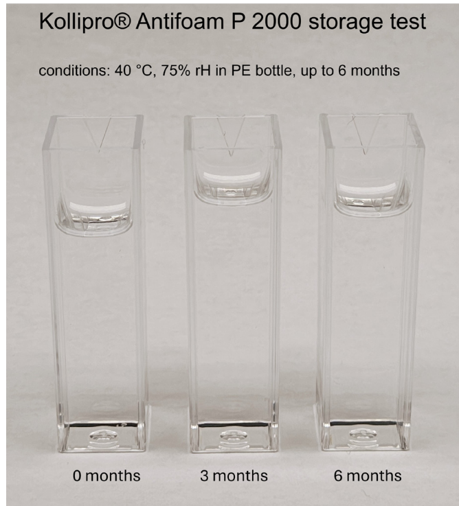
Figure 2: Storage test of Kollipro® Antifoam P 2000 at 40 °C at 75 % relative humidity. Storage was conducted in PE bottles. The product shows no discoloration after 6 months of storage.
