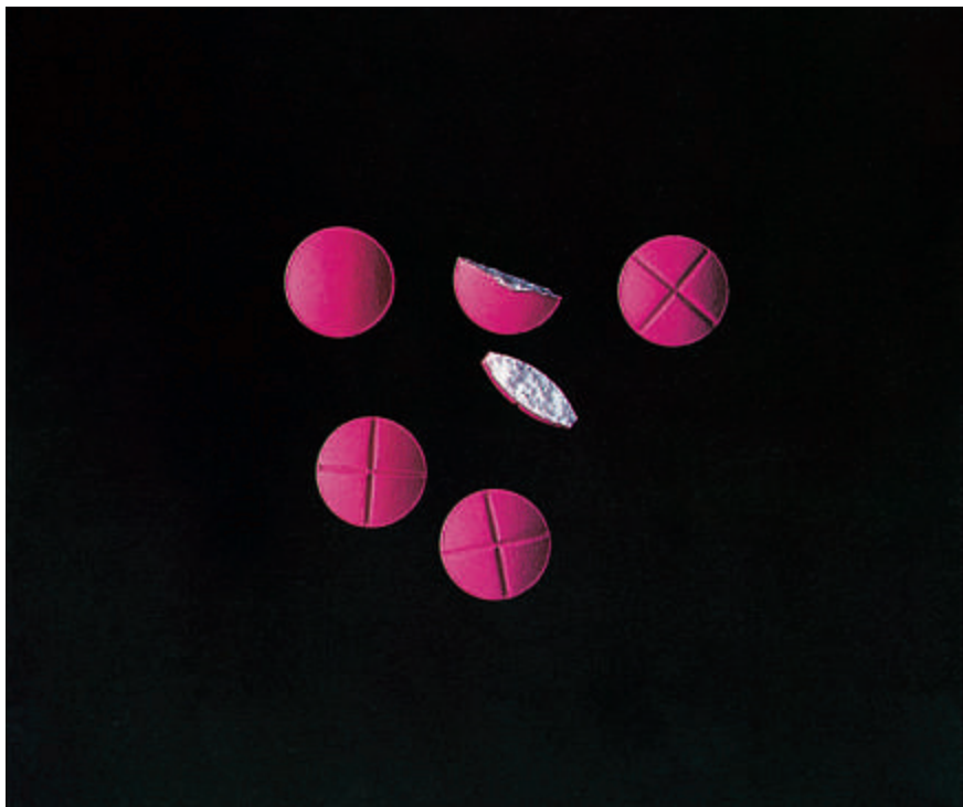
Fig. 4.23: Tablets after sugar film-coating with Kollidon® VA 64 as described in Table 4.28
