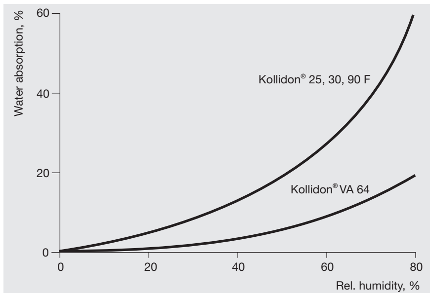
Fig. 4.9: Hygroscopicity of Kollidon® VA 64 and Kollidon® 25, 30 or 90 F for comparison, after 7 days at 25 °C
